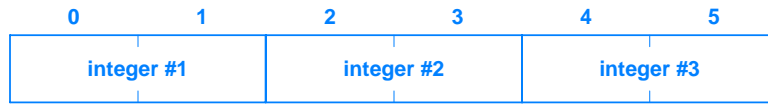
Figure 3.10 A data aggregate consisting of three sixteen-bit integers arranged in contiguous bytes. In the figure, the six bytes have been numbered in big endian order.
