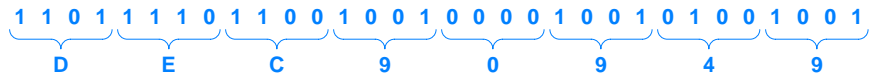
Figure 3.4 Illustration of the relationship between binary and hexadecimal. Each hex digit represents four bits.
