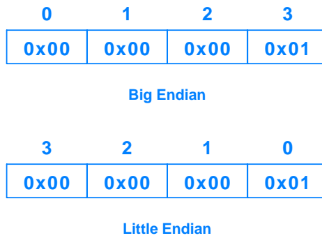
Figure 3.7 Illustration of big endian and little endian byte numbering for a thirty-two bit integer equal to 1. Little endian numbers the least significant byte zero; big endian numbers the most significant byte zero.
