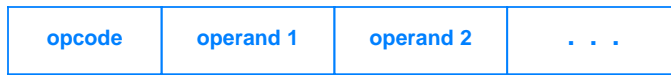
Figure 5.1 The general instruction format that many processors use. The opcode at the beginning of an instruction determines how many operands follow.
