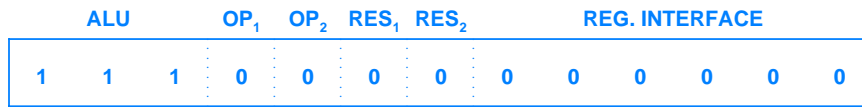
Figure 7.10 An instruction that can be inserted to add delay processing to wait for the ALU to complete an operation. Timing and delay are crucial aspects of horizontal microcode.
