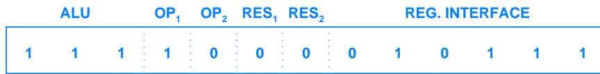
Figure 7.11 An example instruction that simultaneously continues an ALU operation and loads the value from register seven into operand hardware unit one. Horizontal microcode makes parallelism easy to specify.
